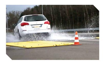
A mechanical device destabilizing even the heaviest vehicles legally on the road, our skid inducer is designed to improve driving techniques.
